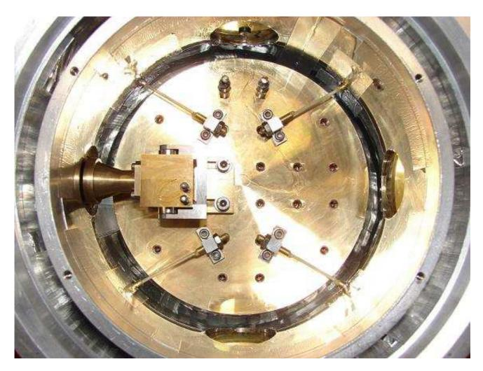
**Photo 1.2b.** The inside view of the tuned InSb detector system
