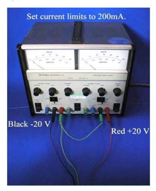
**Photo 5.2.** Power supply connections
