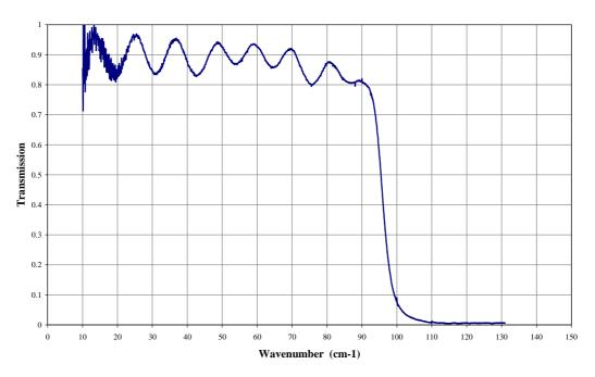
Fig. C1. Transmission spectrum for the type QMMF 100cm<sup>-1</sup> low pass filter
