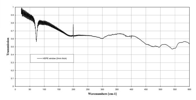
**Fig. C.2.** Measured transmission of a 2mm thick HDPE window from 20cm<sup>-1</sup> to 600cm<sup>-1</sup>. The polyethylene characteristic absorption increase is clearly seen around 73cm<sup>-1</sup>
