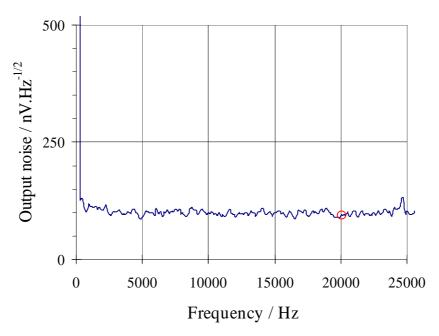
**Fig. 5.1b.** Typical preamplifier input shorted noise spectra Amplifier gain = x100. Noise at  $20kHz = 1.0nV.Hz^{-1/2}$
