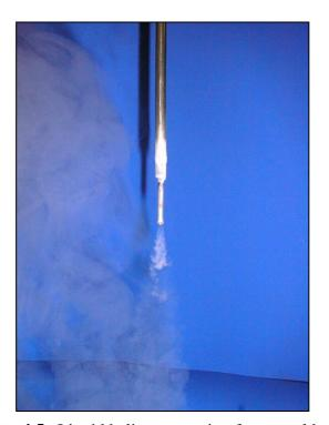
Photo 4.5. Liquid helium emerging from a cold tube
