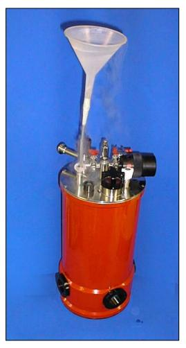
**Photo 3.1.** Using a funnel to fill the cryostat with liquid nitrogen
