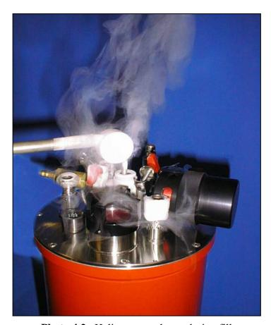
Photo 4.2. Helium gas exhaust during fill
