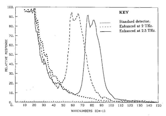
**Fig. A.1.** Spectral responsivity of a QFI/X detector with no magnetic field applied and two examples of type QFI/XB detectors enhanced at 2THz and 2.5THz
