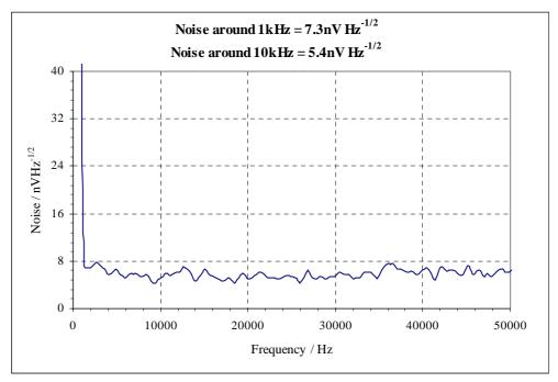
Fig. 6.3. System output noise spectrum for the InSb detector 0 to 50kHz
