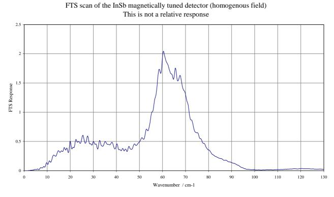
**Fig. 6.5.** Scan of the response of the tuned indium antimonide detector in a Fourier Transform Spectrometer showing the cyclotron resonance peak
