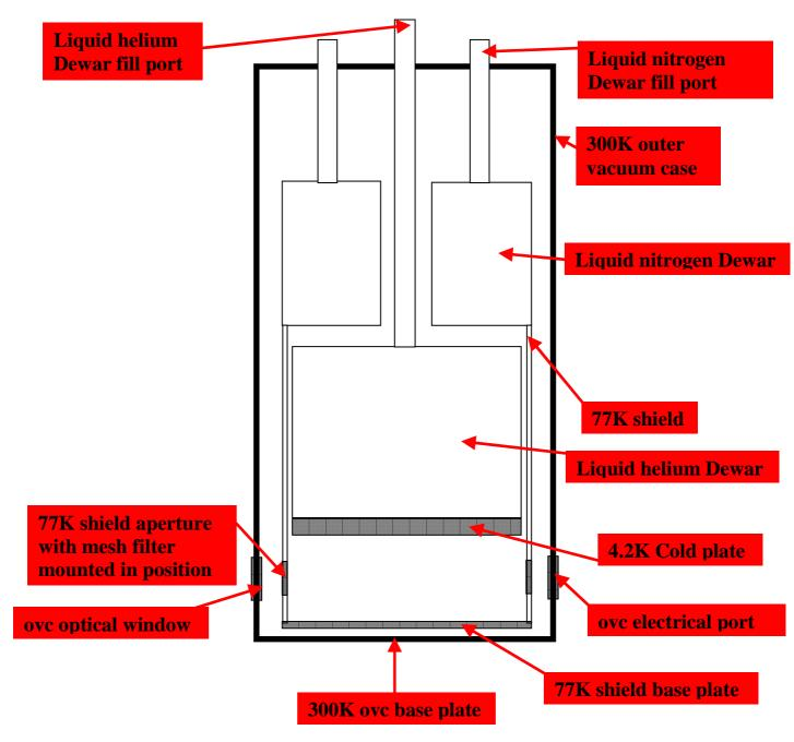
Figure 1.1. Cryostat schematic showing the main features of the cryostat. Not to scale
