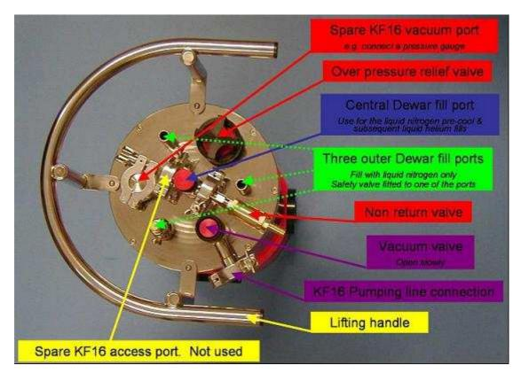
**Photo 2.1.** TK1813 cryostat top-plate fittings
