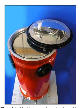
**Photo 1.4.** Liquid nitrogen base-plate in position
