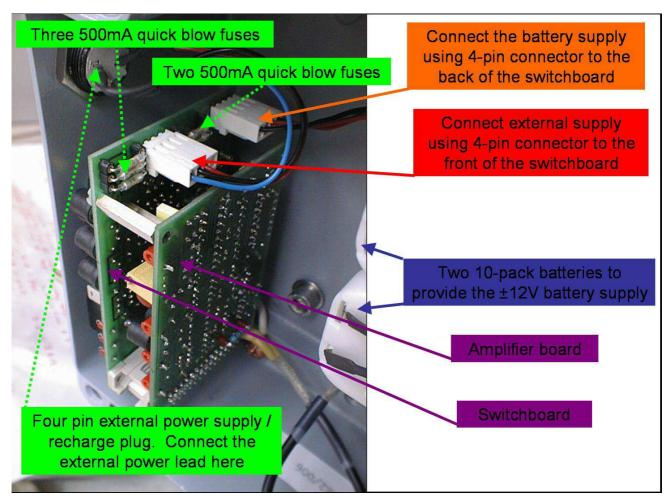
**Photo 5.1b.** The preamplifier boards
