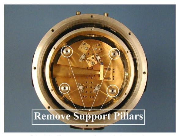
**Photo 1.2a.** The four support pillars and the detector optics
