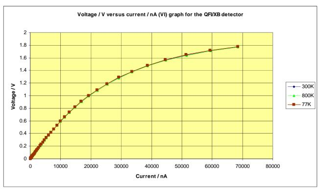
Fig. 6.4. The detector system VI characteristic measured with both a 77K, 300K and a 800K dc load
