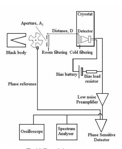
Fig. 6.1. The optical test arrangement
