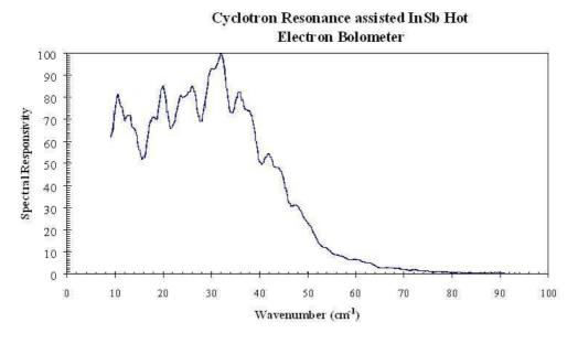
Fig. A.2. Spectral responsivity of the Type QFI/XBI detector
